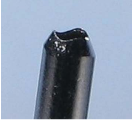
Figure 1. Close-up of the triple-waved tipped extraction needle.
